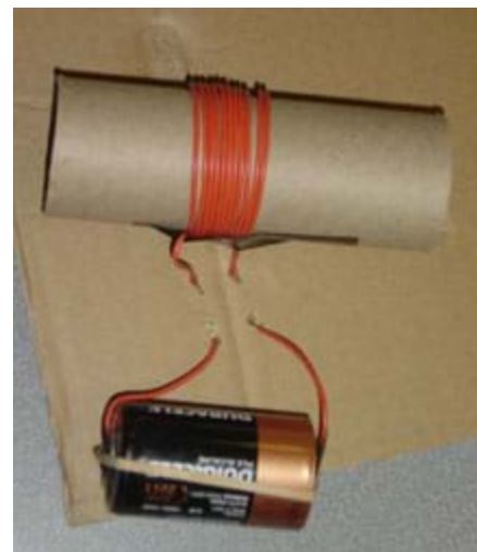
Figure 2. Setup for an Electromagnetic Field Station.
