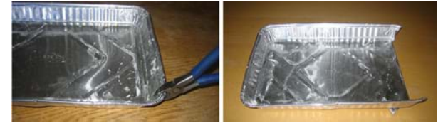
Figure 1. Prepare the riverbed model by cutting the baking pan at two corners and folding under the end flap.
