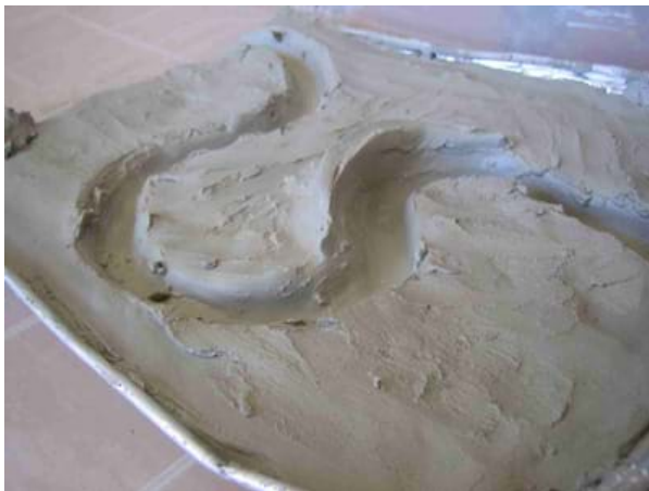
Figure 8. Model of a riverbed with a large curve and levee.
