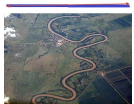
Figure 4. As applied to a river, sinuosity is defined as the path a river takes compared to the shortest possible path that could be taken.
