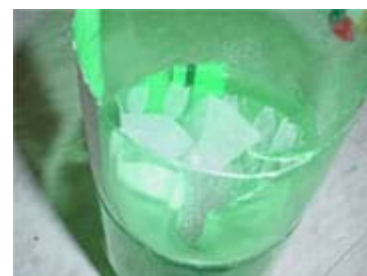
Figure 2. A 2-liter bottle with a coffee filter placed in the bottom.
